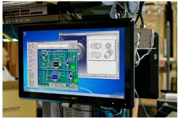
Manufacturing and Industrial environments are notoriously dirty. Dust, metal fragments, and even liquid contaminants can drastically cut short a computer's lifespan on the factory floor. The iPC S series has been engineered with fanless cooling technology and are IP65 rated to prevent any particulates from getting into the unit and damaging internal components.
